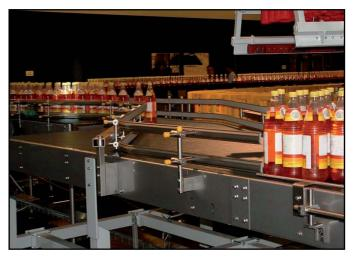
There's also a completely flexible execution that allows a flexible radius or a twisted roller guide.
